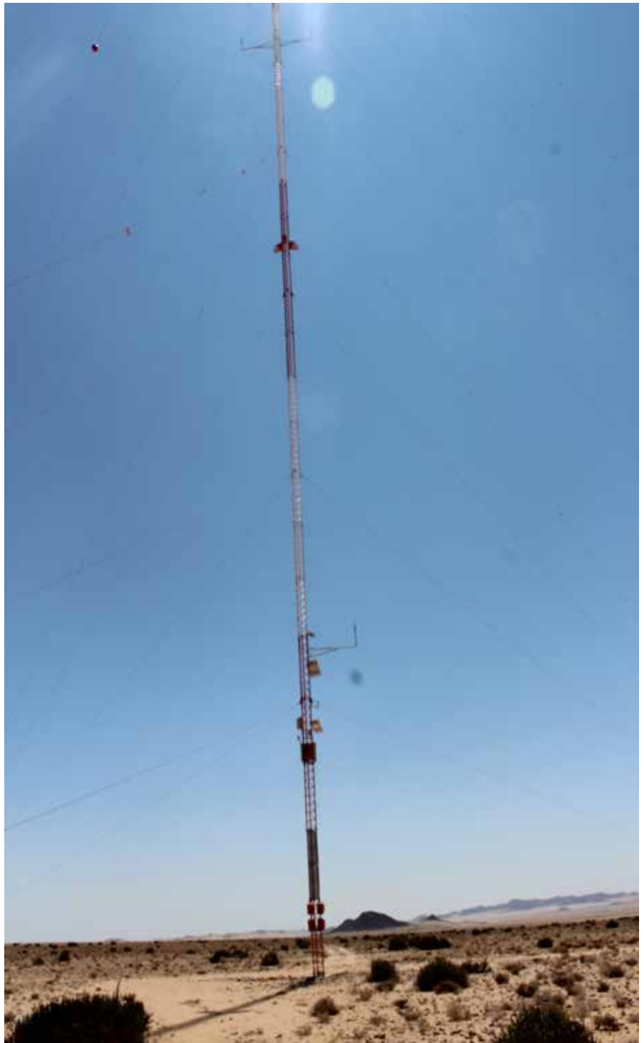
SENSITIVE ENVIRONMENT: One of Hyphen Hydrogen Energy's Meteorological Masts located in Tsau //Khaeb National Park. The masts are wind measuring towers used by to model the energy yield of wind and solar resources in Namibia.
