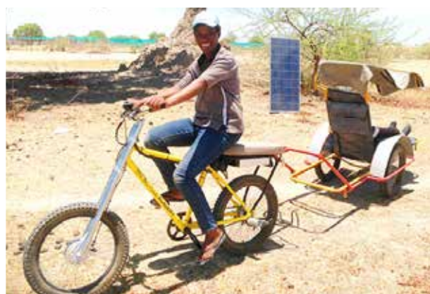
TEST RIDE: Hilya Ekandjo testing one of the solar-powered electric bike ambulances at Okafitu, in the Omusati region
